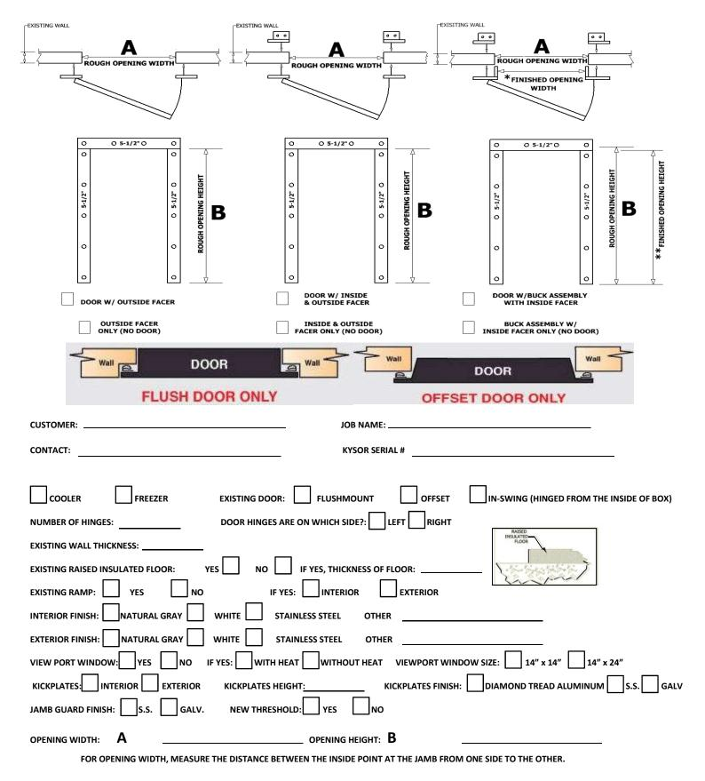
FOR OPENING HEIGHT, MEASURE THE DISTANCE FROM THE FLOOR TO THE UNDERSIDE OF THE TOP JAMB OPENING.
