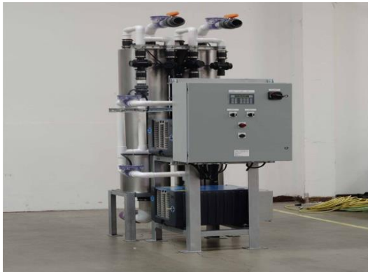
Figure 2 – EVAC condensate vacuum skid with control panel
