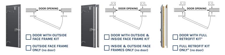
\*NOTE: Once installed, the full retrofit kit will reduce the door opening width by 4" and height by 2".
